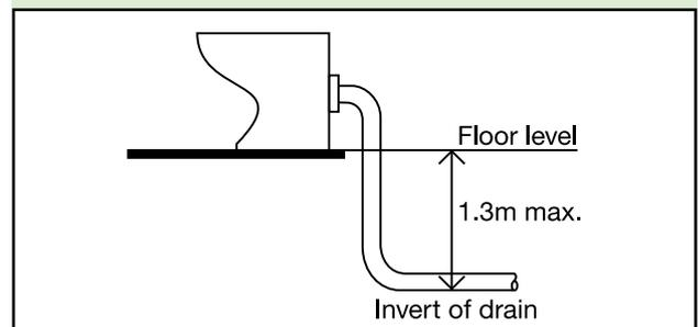
Diagram 2 Branch connection to stacks – crossflow prevention
