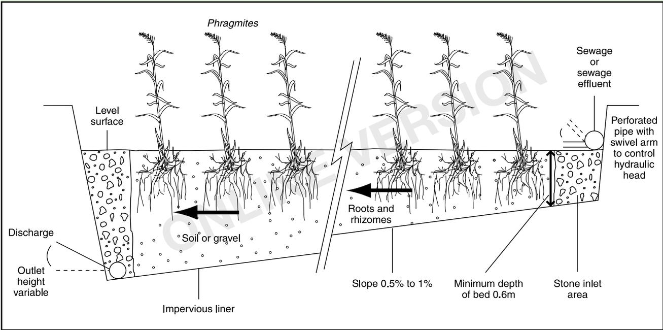
Diagram 4 Typical vertical flow reed bed treatment system
