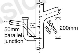
**B** Angled connection or 50mm diameter parallel junction where a branch discharge pipe would enter the WC no connection zone
