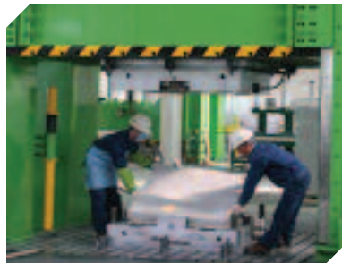
Ejecting Molded Panel After certain period time of molding, take out the molded panel from molds.
