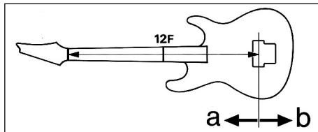
\* Please note that strings can be broken when the saddle is moved, so always loosen the strings before making adjustment.
