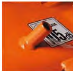
Deck cleaning pipe for connecting water hose
