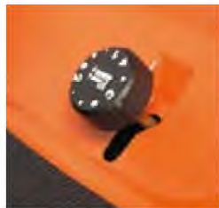
Easy reach cutting height adjustment dial
