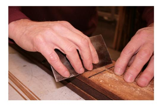
This method of planing is extremely accurate, rod tips may measure only about .060 inches, and therefore an individual tip strip measures a mere .030 of an inch.
