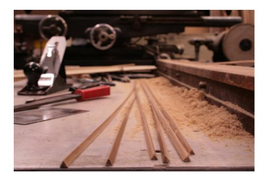
We achieve this uniform configuration by carefully hand planing each strip using a wooden jig which has been set to a 60 degree angle. The resulting uniform strips are non-tapering triangles of uniform length.
