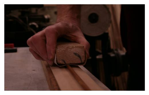
After the glue has cured the string removed and excess glue is sanded, filed or scraped off of the blank. The sections are again straightened and cut to the appropriate length. This is finally the point at which the work begins to resemble a fishing rod.
