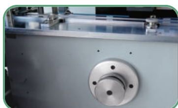
Adjust the size of the label by simply adjusting the turntable to get the desired size.
