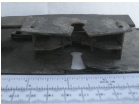
**Difficult to see in this picture, but the bridge ward on the upper right has been bent — this is easily remedied (late 19C stock lock).**
