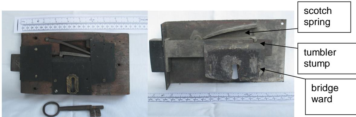
**Banbury stock lock and its distinctive key (left). Stock lock [plate stock lock] late 19C, removed from its stock, looking at the inside keyhole side (right).**
