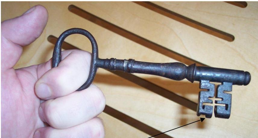
**Keys of this quality should be carefully guarded – they are expensive to replace. This one, c1810, shows wear from the strongly sprung tumbler, the key having been used only from one side. Time to retire this key to secure storage (or display, if the lock is not relied on, e.g. its door cannot be opened from outside) and use a modern replacement.**
