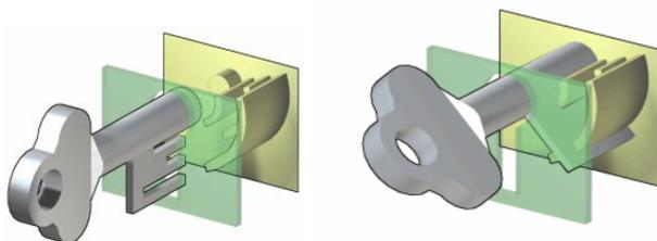
**Two diagrams showing the warded lock principle (in a single-sided lock), using wheel wards.**
