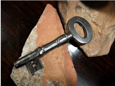
**Broken key — the result of dropping on a hard floor.**
