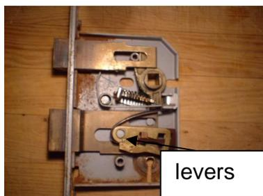
**Basic 3 lever 2-bolt lock (sash lock) suitable for privacy for interior door — UNSUITABLE for exterior doors. This example shows H-shaped (‘Chubb type’) levers.**
