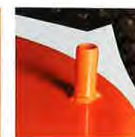
Deck cleaning pipe for connecting water hose
