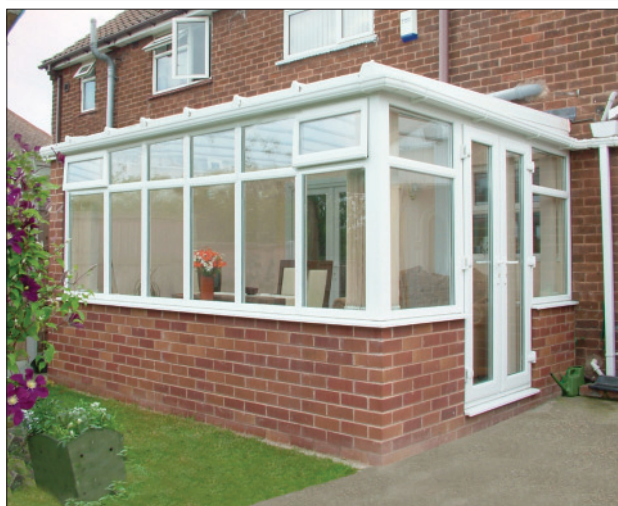
Figure 4 Lean-to style conservatory roof
