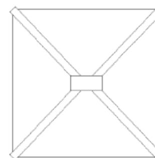
Maximum size Contemporary Pyramid lantern as per line drawing above = 1500mm x 1500mm.
