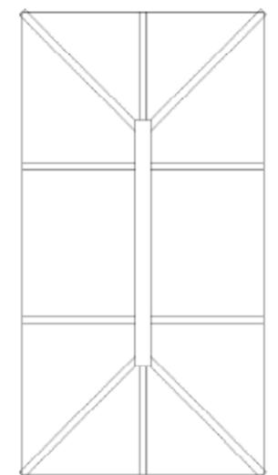
Maximum size Standard lantern as per this rafter layout 3000mm x 4000mm - can go up to 5000mm x 10000mm with additional rafters.
