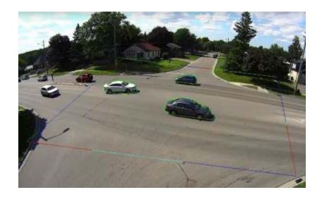
There is no limit to the number of roads and junctions on which traffic can be counted using the scaleable CCTV system. Counts can cover any period of time: the number of cars passing in each hour or each day for example.
