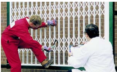
SeceuroGuard 1001 undergoing a simulated attack test.
