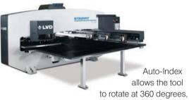
saving the customer any potential expensive tooling charges. Turret punching offers the customer a host of specialist tooling requirements. i.e.; electrical conduit knockouts, recess dimples and various sizes of airflow louvres, plus any bespoke shapes or profiles.
