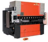
3 off Amada HFE 80-25: 2500mm/80 tonne with automation technology.
