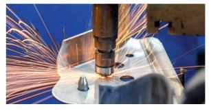
Resistance spot welding (RSW) is a process in which contacting metal surfaces are joined by the heat obtained from resistance to electric current. Work-pieces are held together under pressure exerted by electrodes.
