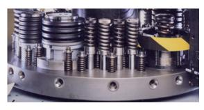
The sheet size/working area is 2500mm x 1250mm with sheet repositioning to increase the working area. A maximum hole diameter single hit of 76mm for 1.5mm thickness material. Our maximum punching capacity is 6mm mild steel or 4mm stainless steel.
