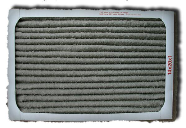
One of the easiest, but often neglected, ways to keep your air conditioning cost down is to make sure your filters are replaced at regular intervals. You should change your **air filter** once a month or as needed based on the manufacturer's recommendations. Several highly efficient filters are available that can extend the useful life.
